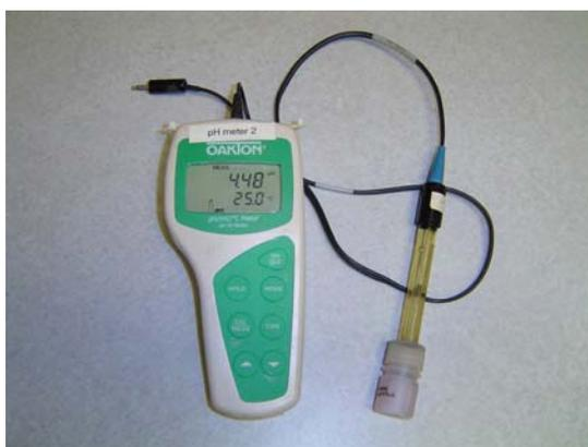
Figure 17. pH meter with electrode
