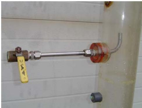
Figure 20. Adjustable sampling port to measure sand concentration
