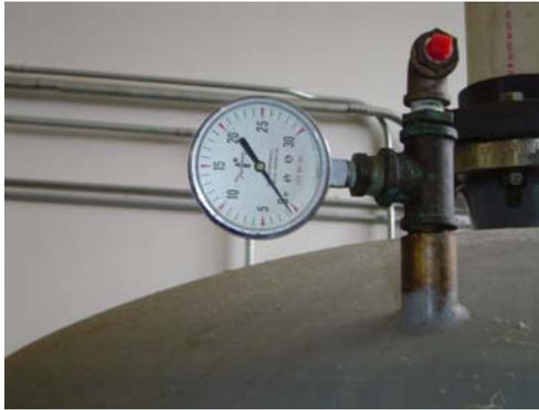
Figure 18. Calibrated pressure gauge attached to the tank
