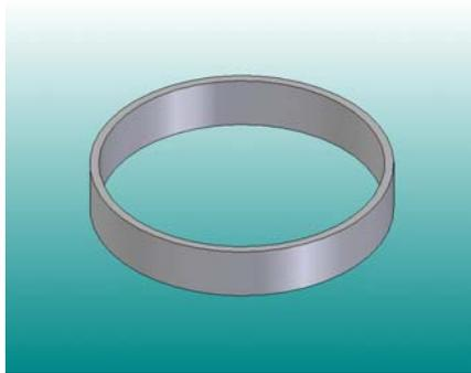
Figure 1 Large ring, used in the larger pipe section (I.D = 4 inch, O.D = 4.25 inch, width = 0.75 inch)
